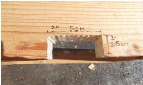
3. Keep sawing out the small sections until it leaves an exit hole 5 cm wide and 2.5 cm high.
