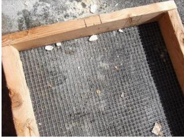
1. With the ICU screen on the ground and wood facing up, measure a 5cm wide section in the middle of one side of the ICU.
